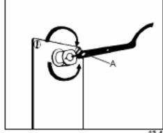
Resecure the combination change plug assembly by screwing it in clockwise with the DF-59 key — do not overtighten (see figure 13-6). Remove the key and store it in a secure area with these instructions and the spanner wrench.
