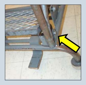
Check joints for loose or missing bolts and for broken welds.
