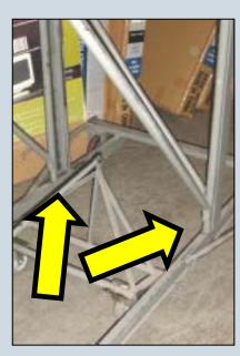
Check joints for loose or missing bolts and for broken welds.
