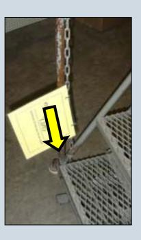
Check the hand rails by carefully climbing the ladder and checking for movement in the handrails.
